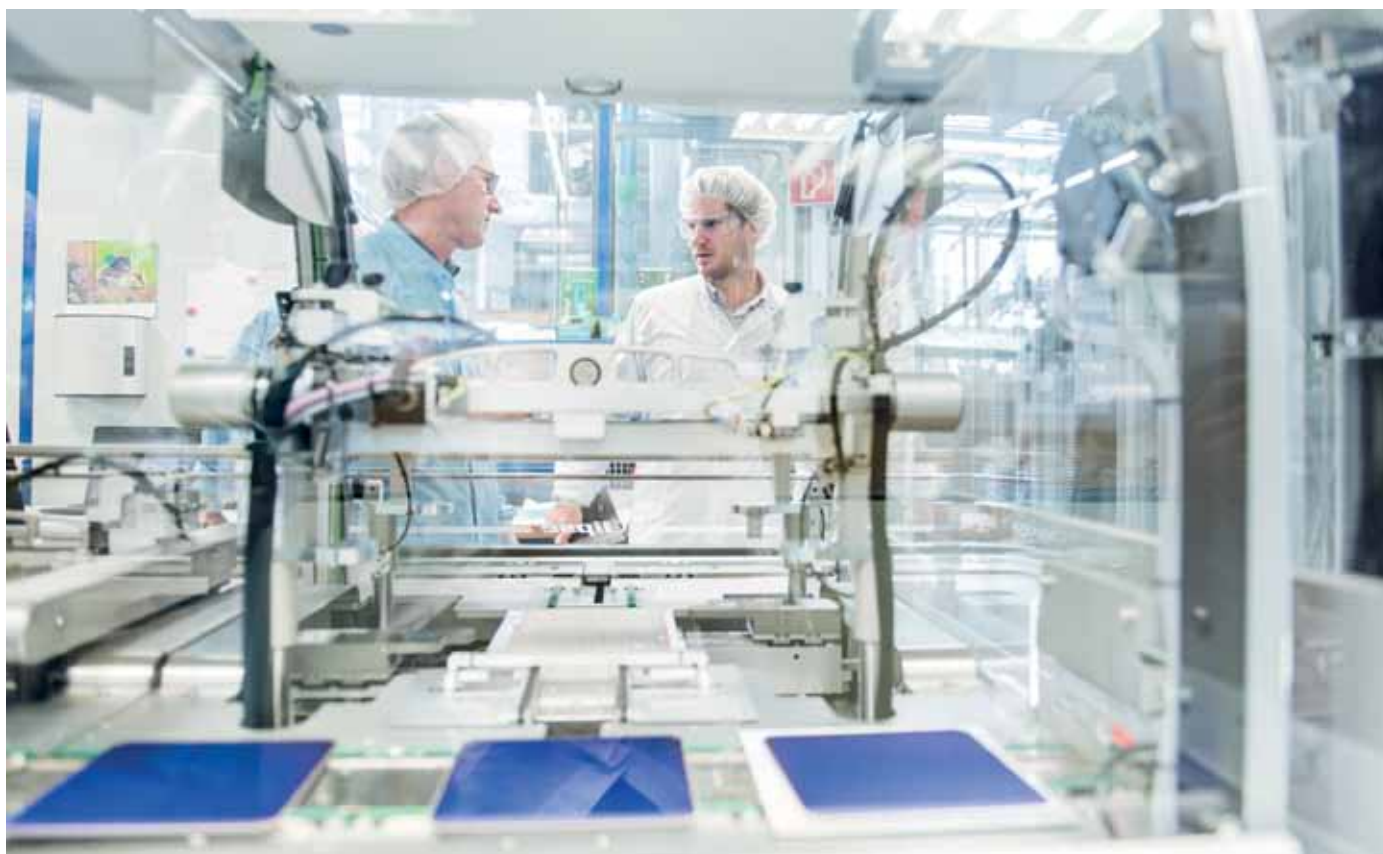
At its Technology & Product Center in Hohenstein-Ernstthal, Germany, Meyer Burger is operating a demo line of its heterojunction technology with a capacity in the low double-digit megawatt range. It reports that running pilot lines is crucial when convincing manufacturers of the stability of new processes.
