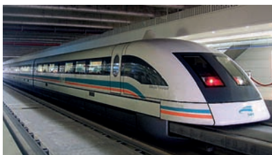
Travelling at a speed of up to 450 km an hour, Shanghai's Transrapid magnetic levitation train covers the 30 km route between Longyang Road Station and Shanghai Pudong International Airport in around 7 minutes 18 seconds, carrying up to 440 passengers.
